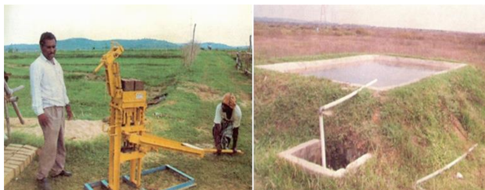
Figure 5.6. Manual soil block press for making mud blocks and tank with mud block and low-density polyethylene film. Source Chowdhury et al. (2016)
